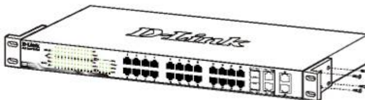
Figure 2.2 – Attach the mounting brackets to the Switch
